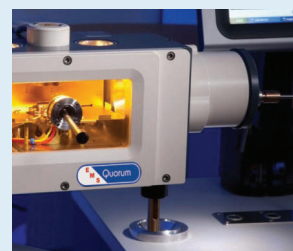
Cryo preparation chamber with cryo transfer device fitted
