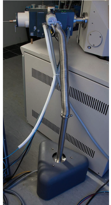
Remotely mounted turbomolecular pumping system
